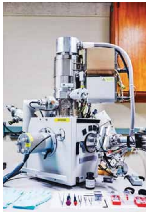
Top right: These discs are used to store nanoscale lattices. Bottom right: A scanning electron microscope has an arm that can compress and bend nanostructures.
