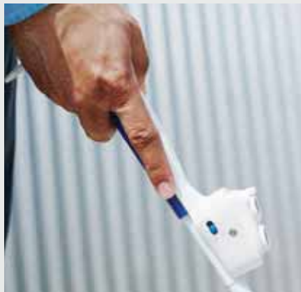
The device vibrates in patterns that indicate the distance to obstacles.
