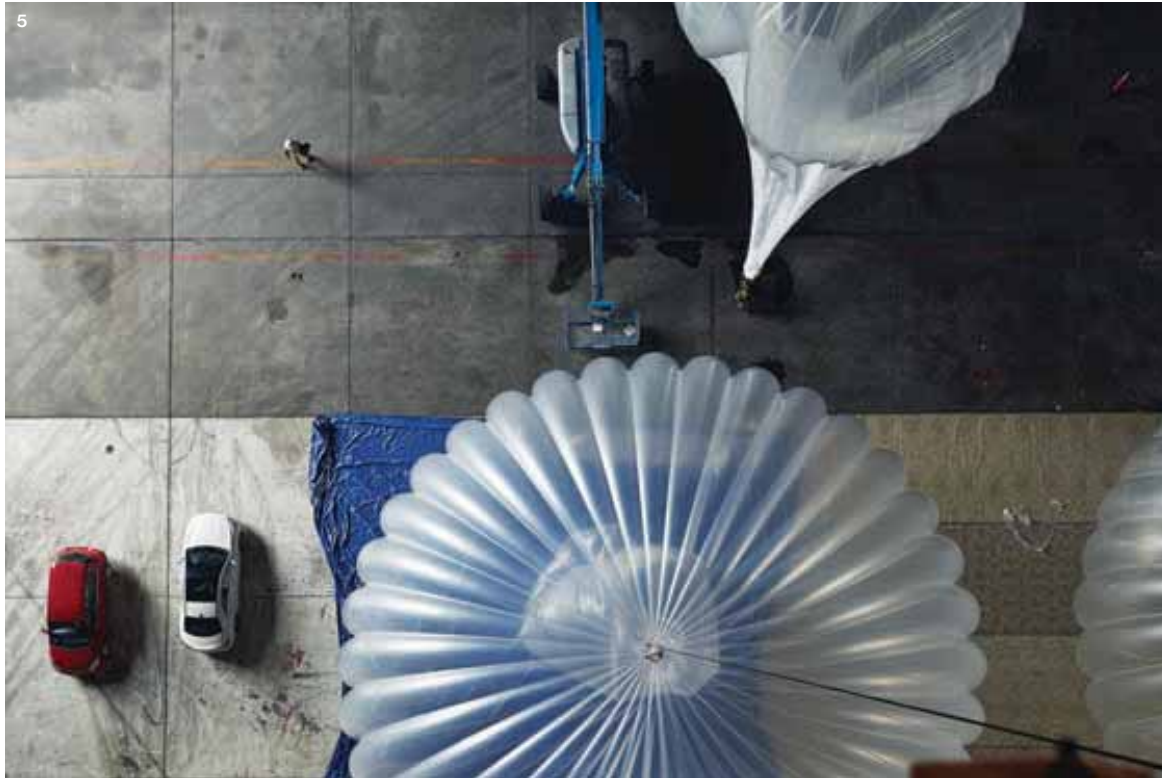
5 Among the upgrades Google is testing for its balloons (seen here from the rafters): using hydrogen, which is cheaper than helium, and having a motor move their solar panels to track the sun.
